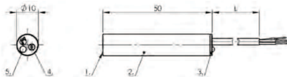
1) Sensing surface, 2) Housing, 3) Cover, 4) Potentiometer, 5) LED function indicator
